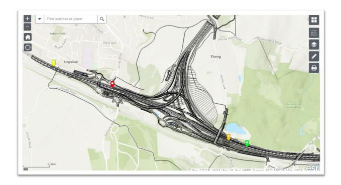
41. From left to right - The yellow marker shows where the lane markings separate the road with just 2 lanes to the right for the A2, and the 2 lanes to the left for local access and LTC access routes. The red marker is where the A2 would become just 2 lanes. The orange marker shows where the A2 becomes 3 lanes, and the green marker where the A2 would be back up to 4 lanes.
