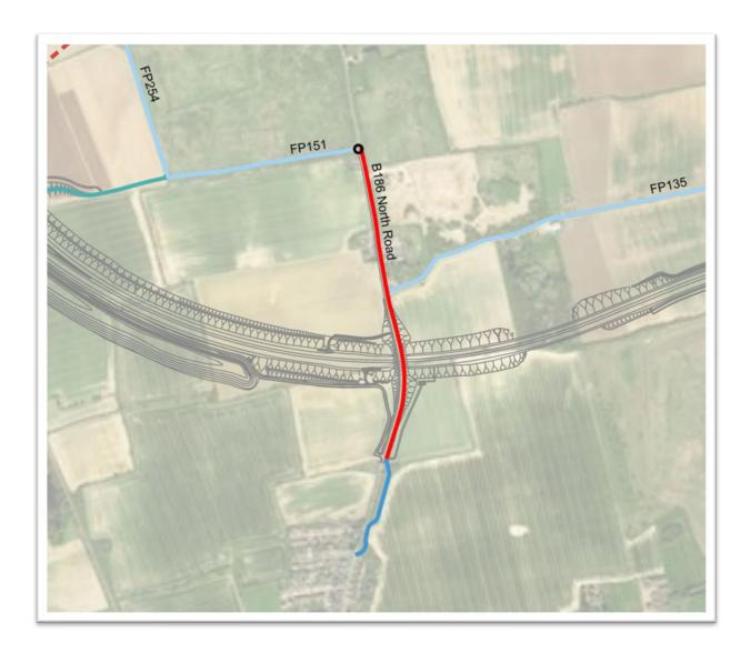
215. This can also be seen in Sheet 39 of 2.5 General Arrangement Plans (Volume C) (Sheets 21 to 49) [APP-017] which further details which side of the road the WCH path runs. It even appears to show that it crosses the road, despite there being no safe crossing at this location. We have screen captured and pasted below the section to help highlight this.
